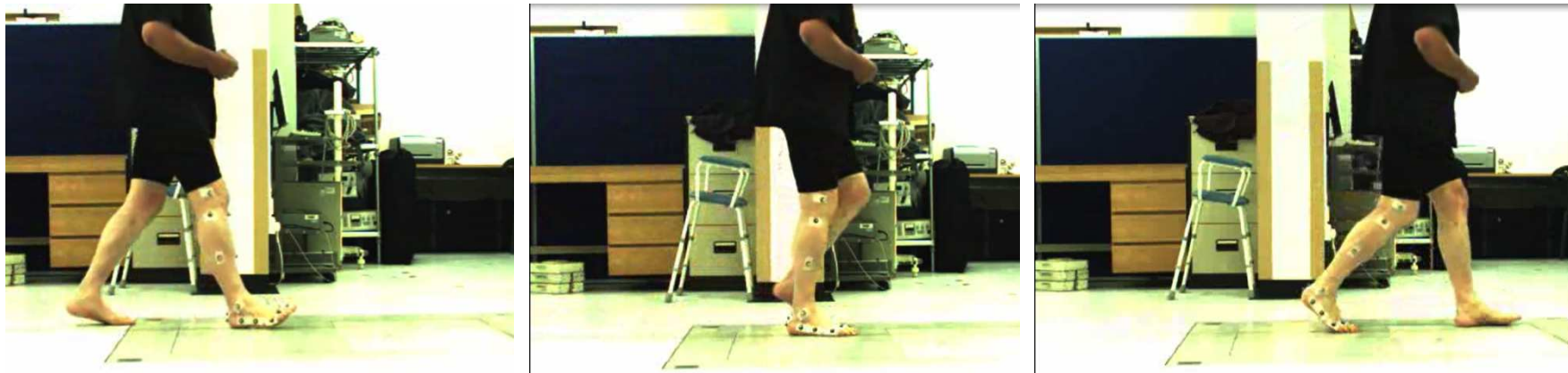
Figure 3.4 Participant walking through the three different stages of the stance phase of gait ( i.e heel strike, midstance and push-off) during gait data capture. Reflective markers placed using the modified OFM method.
