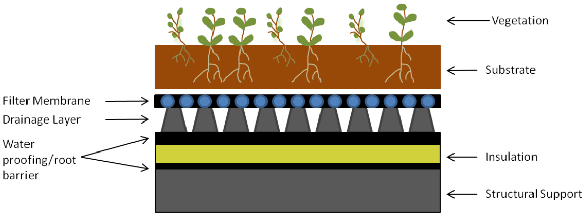
Figure 1.4: a) Small scale model of a standard extensive green roof. b) Cross Section of a Standard Extensive Green Roof (adapted from Oberndorfer et al. , 2007). Photo by Thomas Young, University of Sheffield.
