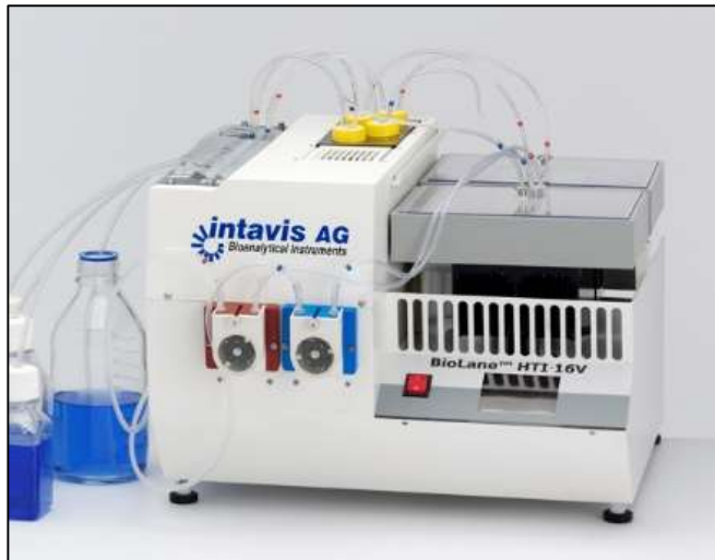
Figure 2-5: Biolane Robot for automated an olig2 in situ hybridisation
