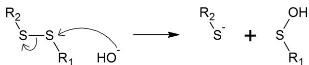
Figure 14: One of the possible mechanisms of disulphide bond cleavage in alkaline media 81
