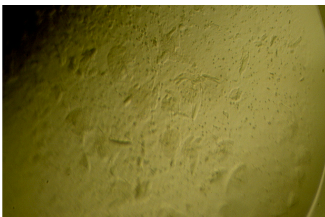
Figure 92. Crystallization of tetramer TSWV N selenomethionine protein using the sitting drop vapour-diffusion method at 25 °C, and crystals were seen in condition 62 from the Index crystallization screening kit (Hampton Research).
