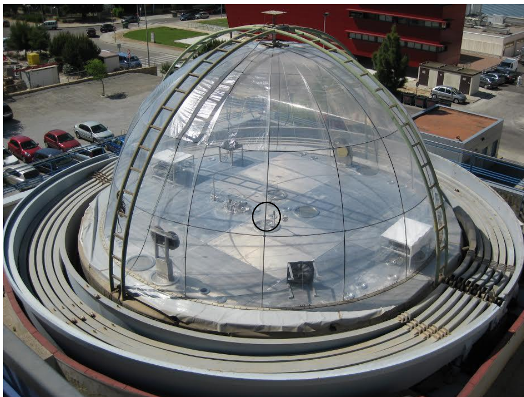
Figure 3.2 - EUPHORE simulation chamber. Black circle displays the PILS sampling inlet, discussed in Section 3.2.2.
