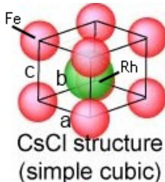
Figure 11: Demonstration of the CsCl-type structure of iron-rhodium. The lattice parameter ( $a = b = c$ ) at room temperature is 2.987 Å. The lattice parameter changes to 2.997 Å above the transition temperature.
