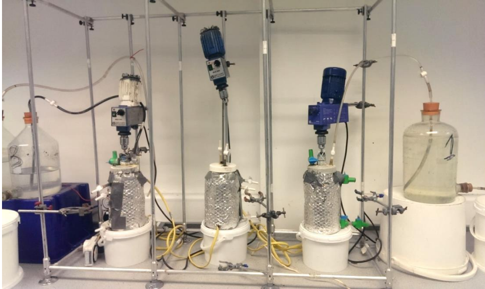
Figure 5.9 CSTR systems during the operation of co-digestion experiments
