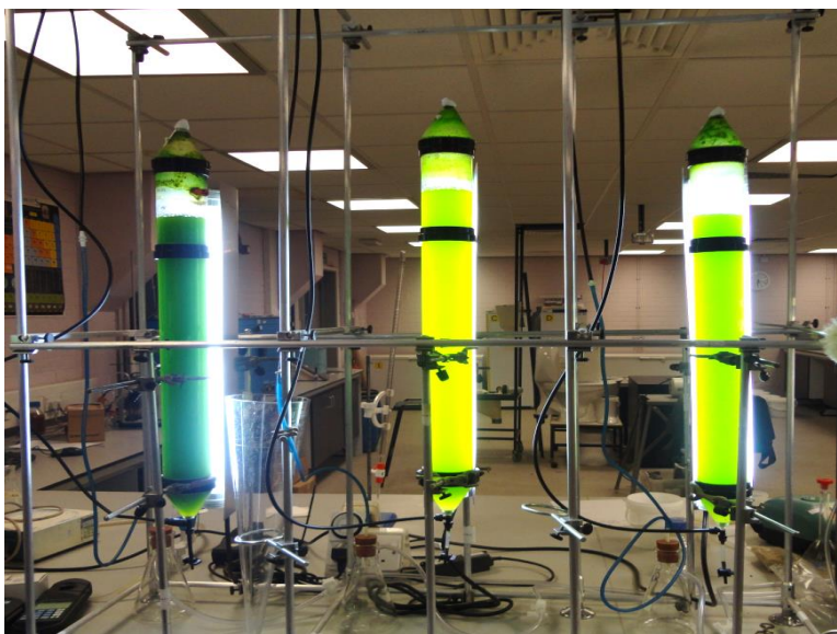
Figure 5.3 Chlorella vulgaris culture in tubular photobioreactors
