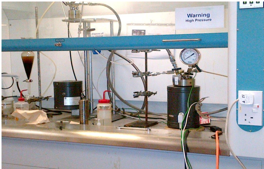
Figure 5.8 Laboratory scale hydrothermal reactor
