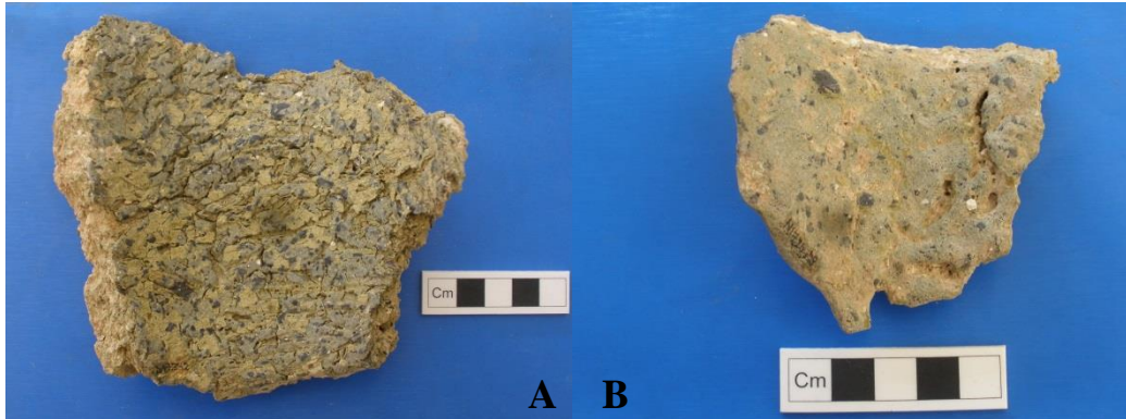
Figure 7.19: Kiln lining from Nemea. (A): vitrified lining from East Stoking Chamber (Sample 267); (B): vitrified lining from kiln fill (Sample 266).
