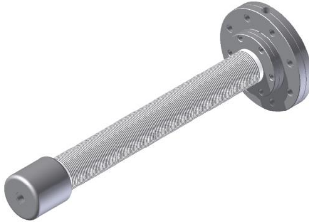
Figure 3.5: CAD drawing showing the electrode mounted on the ribbed ceramic mount and 2.75" CF flange, and attached to the 4.5" degassing flange.
