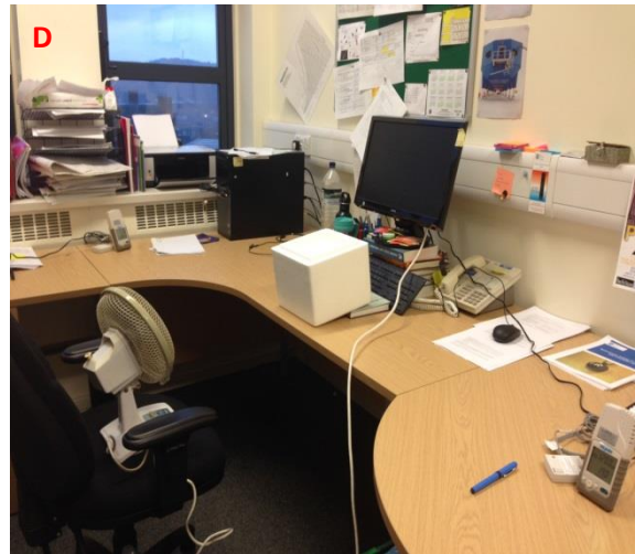
Figure 6-1: Photographs of test office showing some logger locations (A-C) and dry ice with fan (D)
