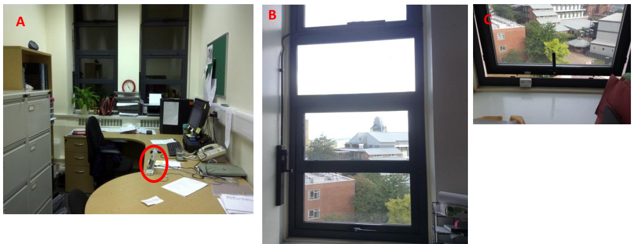
Figure 6-5: Photographs of the windows and the data loggers in a typical office used for the experiment: A – Test office with environmental data logger B – Lower and upper windows and chain opener for upper window; C – State logger on lower window
