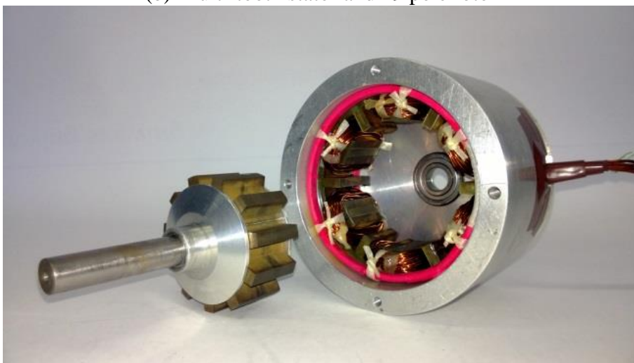
(c) E-core stator and 11 pole rotor
