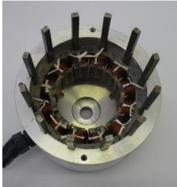
(b) SFPM stator with FAs in all stator teeth
