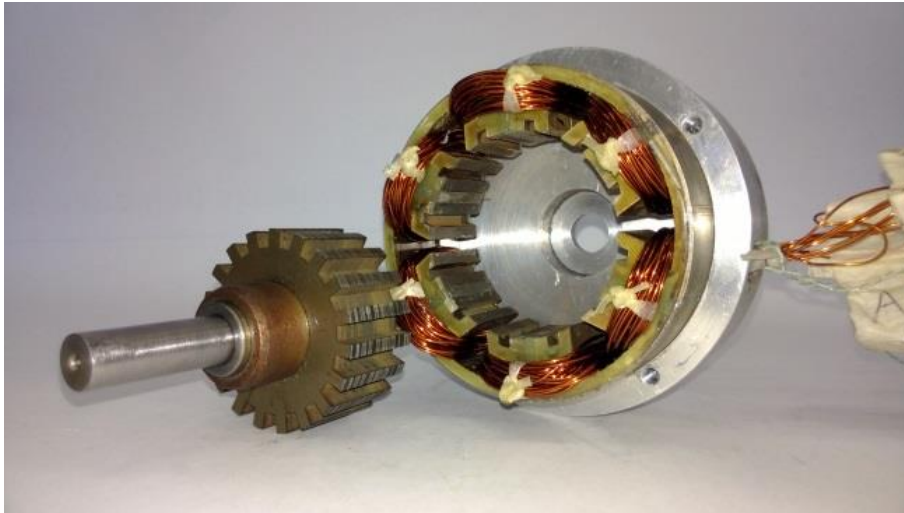
(b) Multi-tooth stator and 19 pole rotor
