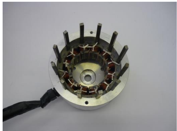
(b) SFPM stator with FAs
