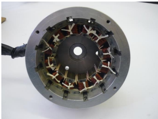
(a) Prototype of 12 pole stator SFPM 10 poles 13 poles 14 poles
