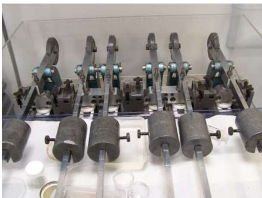
Figure 2.6 – The fully assembled 6 station pin-on-plate wear rig. The top image shows one individual station with the pin submersed in 25% (v/v) bovine serum. The bottom image shows the six stations, each with a cantilever arm and a weight situated to apply 160N of force.
