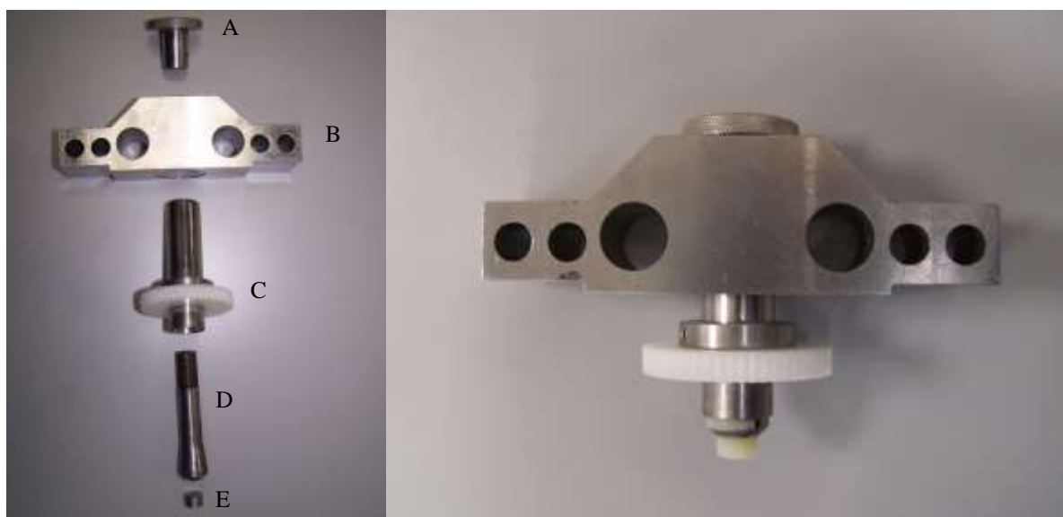
Figure 2.5 – The left hand image shows an exploded view of the components that make up the pin holder. The right image shows the fully assembled pin holder, showing the pin protruding from the bottom and the cog positioned above the pin. The pin holder was composed of the following components; A – Threaded nut; B – Bridge section; C – Pin holder outer sleeve with polymer gear wheel attached; D – Collet (pin holder); E – Spacer pin. The fully assembled image shows a 1050 Vit E 10 UHMWPE pin in place, protruding from the bottom of the pinholder.
