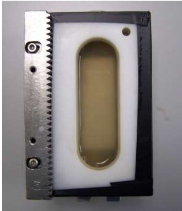
Figure 2.4 – A bird’s eye view of the assembled linear bearing tray and bath with 50 ml of 25% (v/v) bovine serum. The bottom of the image shows the front of the linear tray, where the connecting rods slot in to attach to the tray. The toothed rack is shown on the left hand side of the image. The black PVC tape used to seal the bath is also shown.
