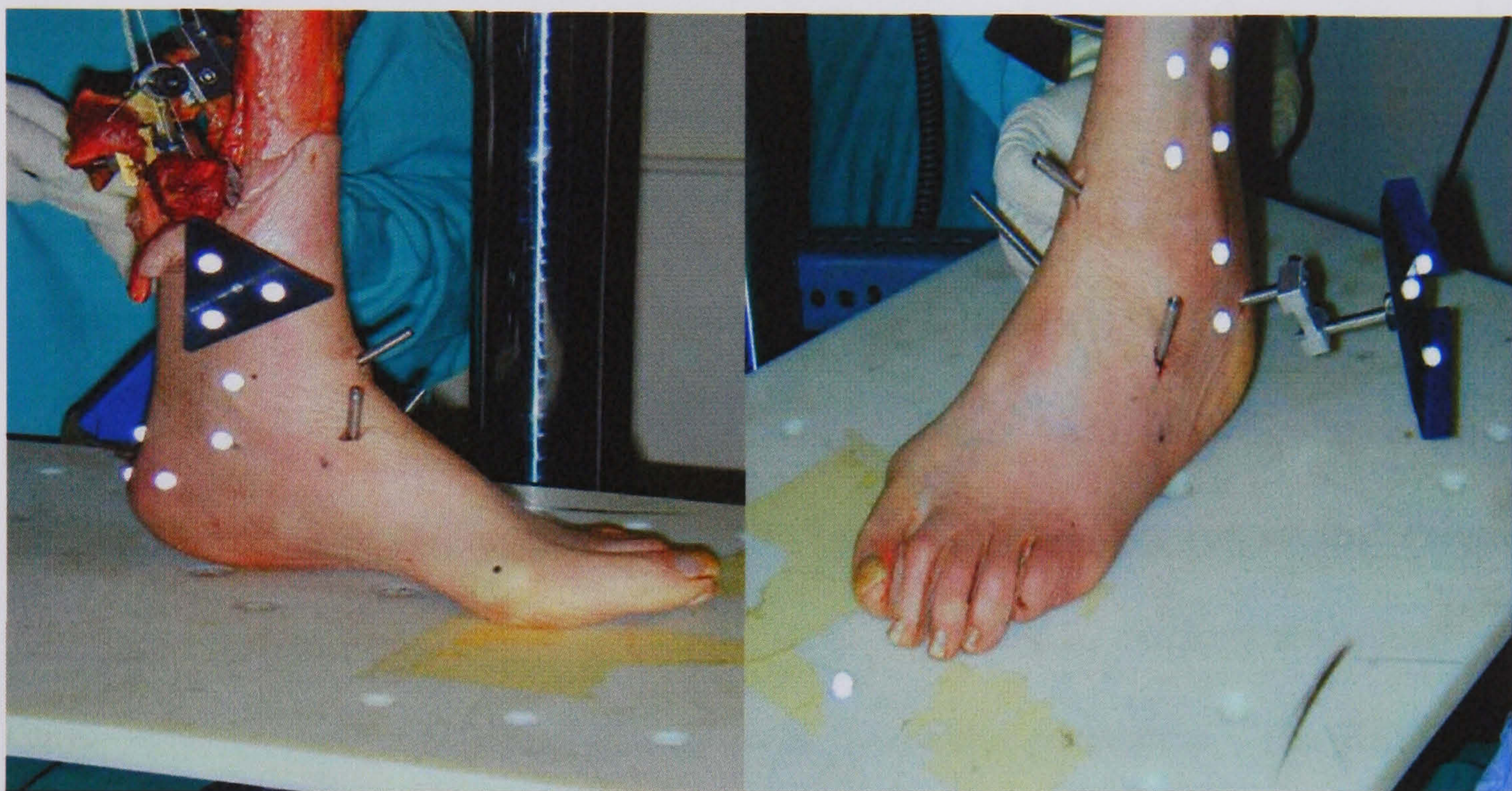
Figure 5.2. Marker setup for the skin vs bone markers experiment. The markers on the triads were used to track the motion of the bones.
