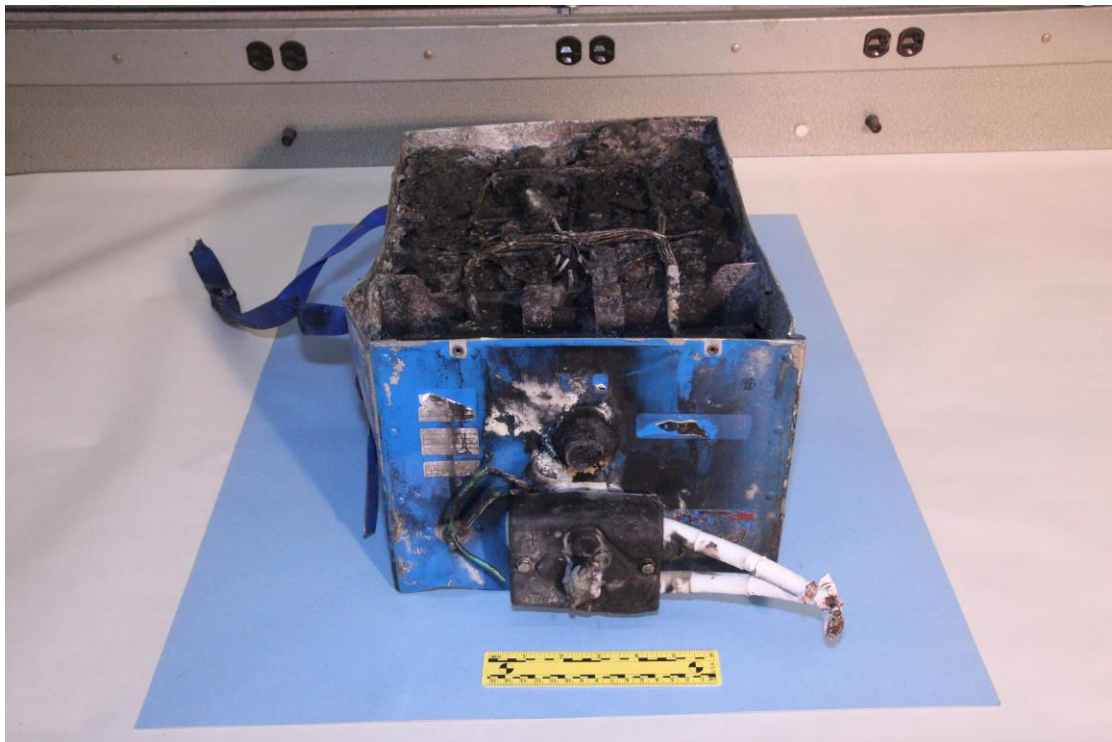
Figure 1.2- NTSB photos of the burned auxiliary power unit battery from a JAL Boeing 787 that caught fire on Jan. 7 at Boston's Logan International Airport.
