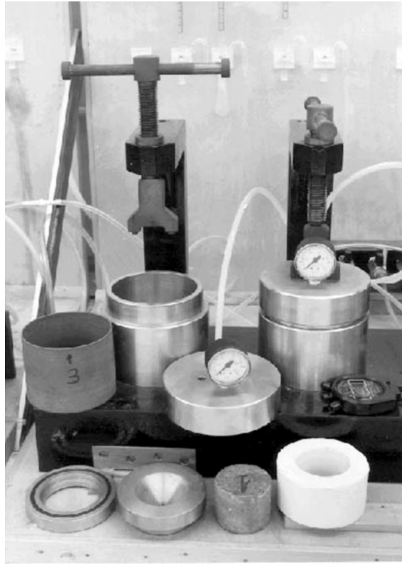
Figure 3.10 Leeds gas permeameter (Image from [354])
