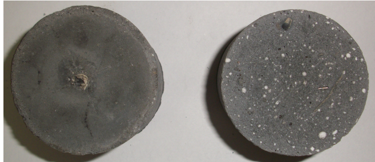
Figure 3.12 Sample as cast (left) and after exposing internal pore structure (right)
