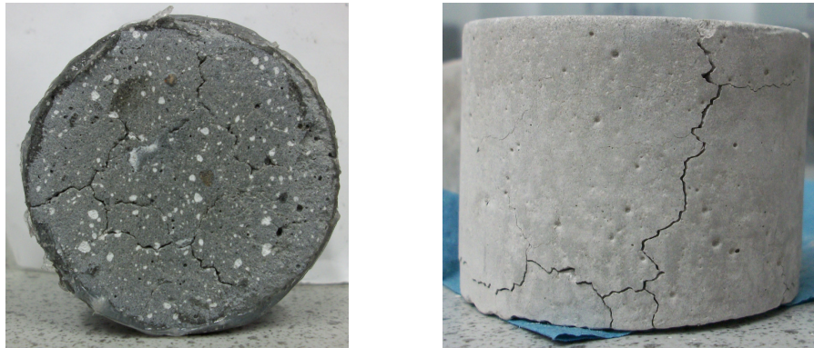
Figure 3.13 Examples of sample cracking after oven drying (left) and freeze drying (right)
