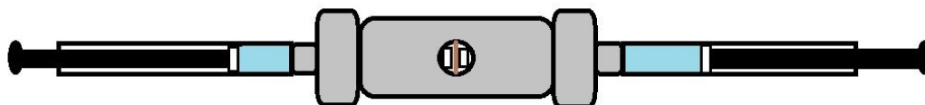
Figure 3. LiposoFast™ extrusion device consists of two glass gas-tight syringes that are attached to a metal chamber containing a polycarbonate membrane. A polymer aqueous solution is passed through the membrane several times in order to obtain more homogenous vesicle sizes 23 .
