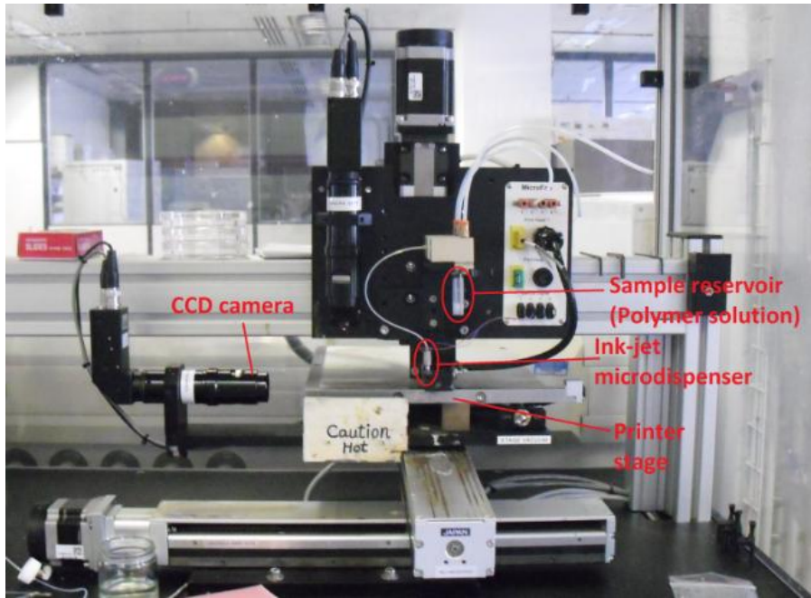
Figure 1. The inkjet printing equipment used in the experiments. The glass slide is placed on the printer stage where the camera on the left is used for imaging during printing.
