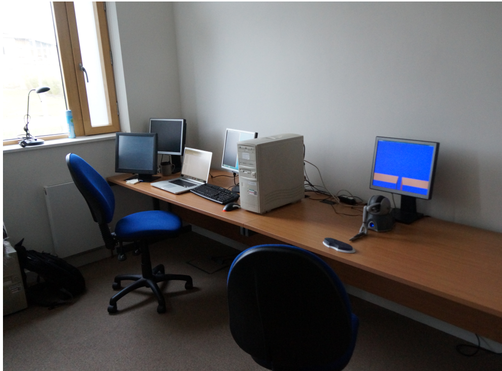
Figure 35 Experiment setup. Far left is the experimenter corner where participant responses were recorded in a MS Excel sheet and trial order was controlled. The right corner is where the participants made the magnitude estimations using the Geomagic® Touch™ FFD.
