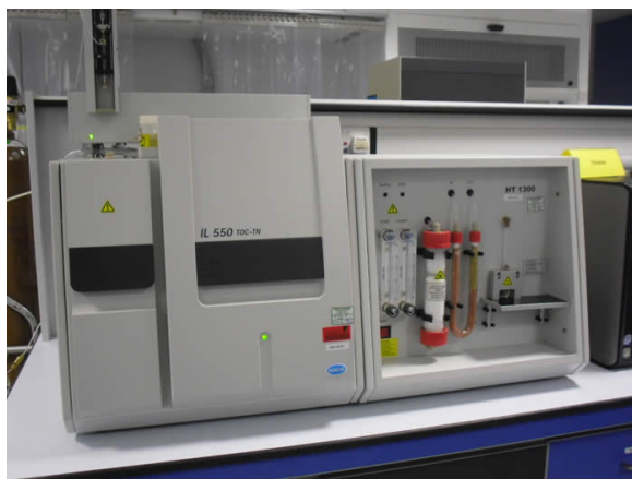
Figure 3.6 Total Organic Carbon (TOC) and Total Inorganic Carbon (TIC) Analyser (Hach-Lange IL550)
