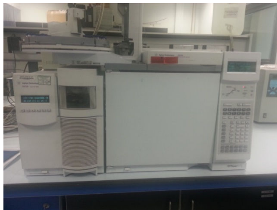
Figure 3.9 Agilent GC-MS used for analysis of FAME content in algae oil
