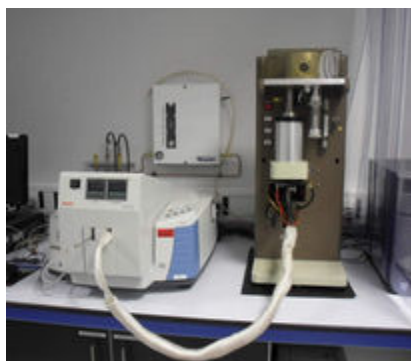
Figure 3.7 Stanton TGA used for thermogravimetric analysis of biomass and oil samples
