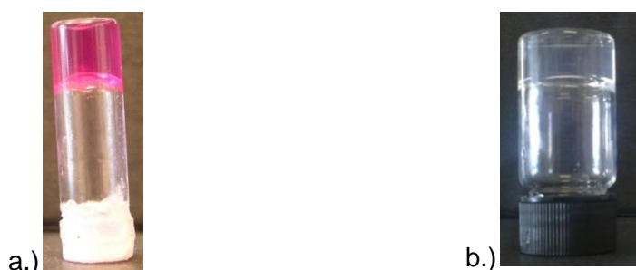
Figure 98 - P_{11-9} self-supporting gel, 20 mg/ml (14 mM) 1 month old a.) in DMEM cell culture medium, b.) in PBS
