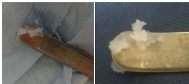
Figure 112 - Waxy residue of P 11 -8 gel after liquid phase is removed upon cleaning of the rheometer.
