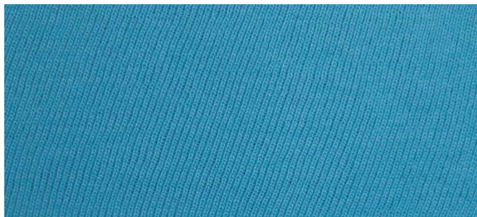
Figure 2.4 Knitted sample number 2.23 with a mean colour difference of 15 CIELAB \Delta E (1:1 scale)
