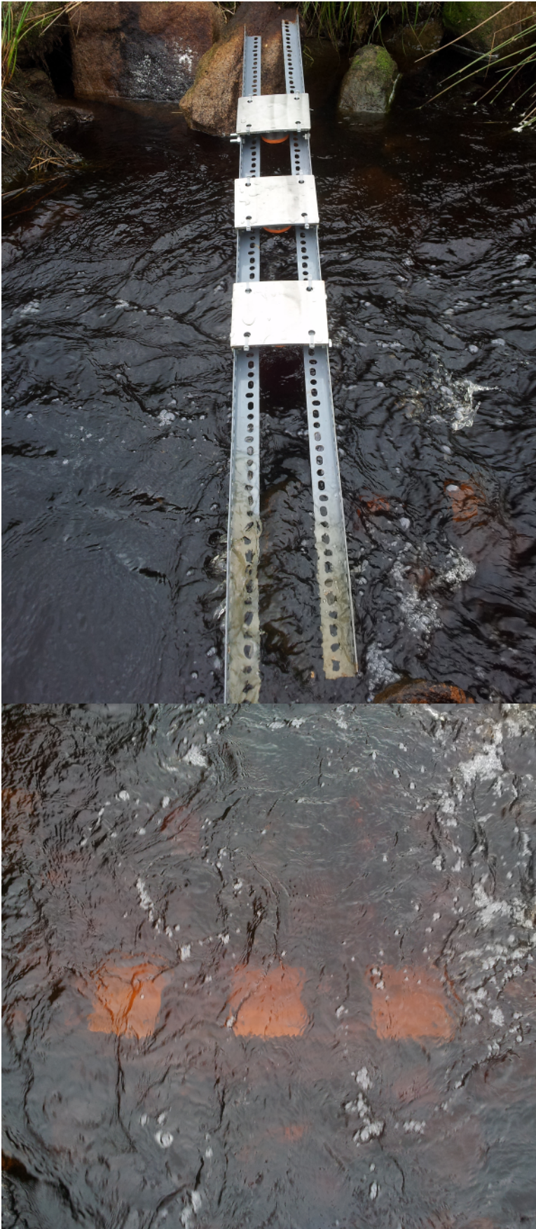
Figure 7.2: Impact sensors mounted on frame (top) and installed in stream (bottom).
