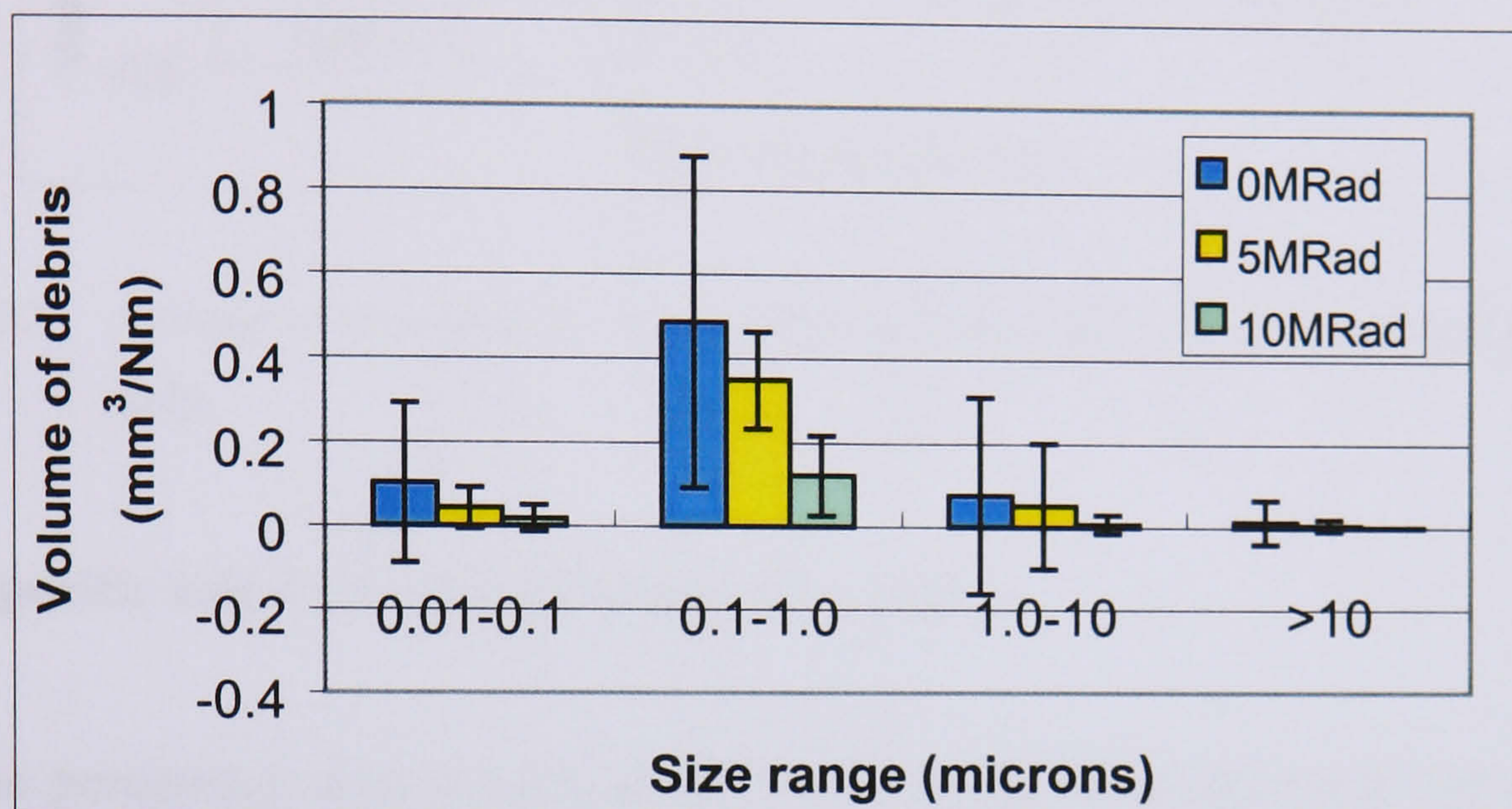
Figure 5.31 Volume of wear particles in the different size ranges from the smooth pin on plate study.
