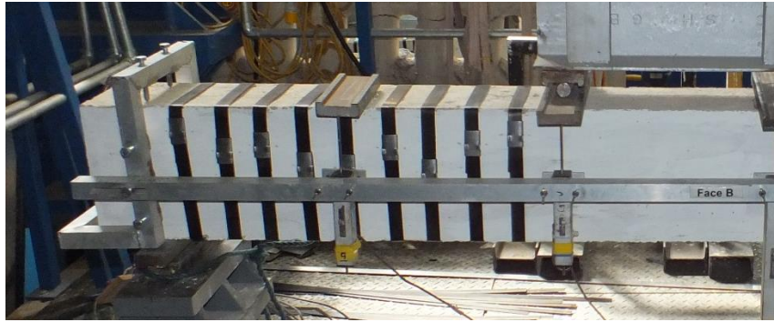
Figure 3-10 External metal strapping positioned along the ‘strengthened side’
