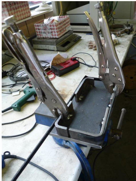
Figure 3-4 Manufacturing of the GFRP shear link
