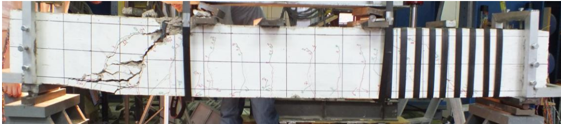
Figure 4-50 Shear failure of GB52-P80
