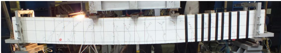
Figure 4-4 GB50-P80 at the loading of 60 kN
