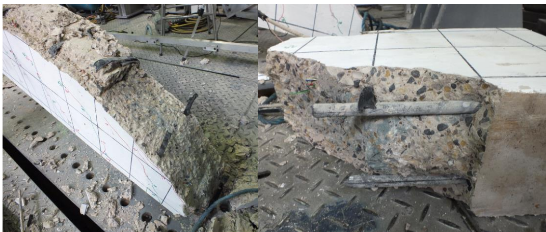
Figure 4-28 Diagonal failure of CB51-P150
