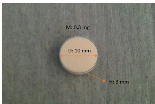
Figure 4.1 Compressed sodium carbonate tablet
