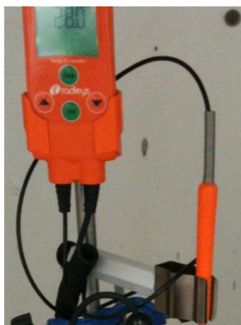
Figure 4.4 Temperature controller of stirring hot plate
