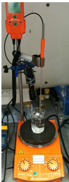
Figure 4.3 Stirring hotplate used for dissolution experiment
