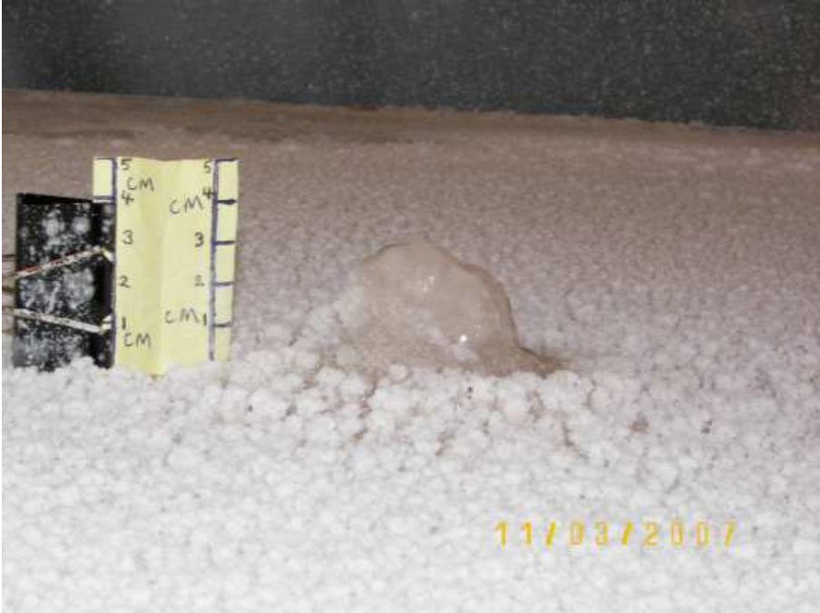
Figure 1.14: 8 Molar sodium nitrate precipitation after 3 day.
