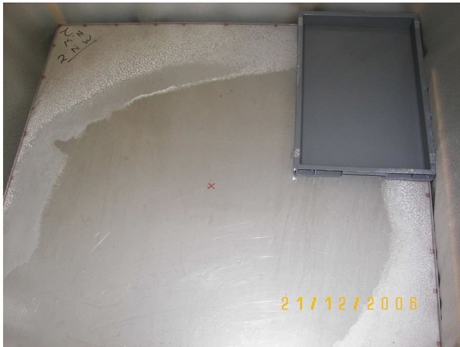
Figure 1.11: 1 Molar sodium nitrate precipitation after 1 day.
