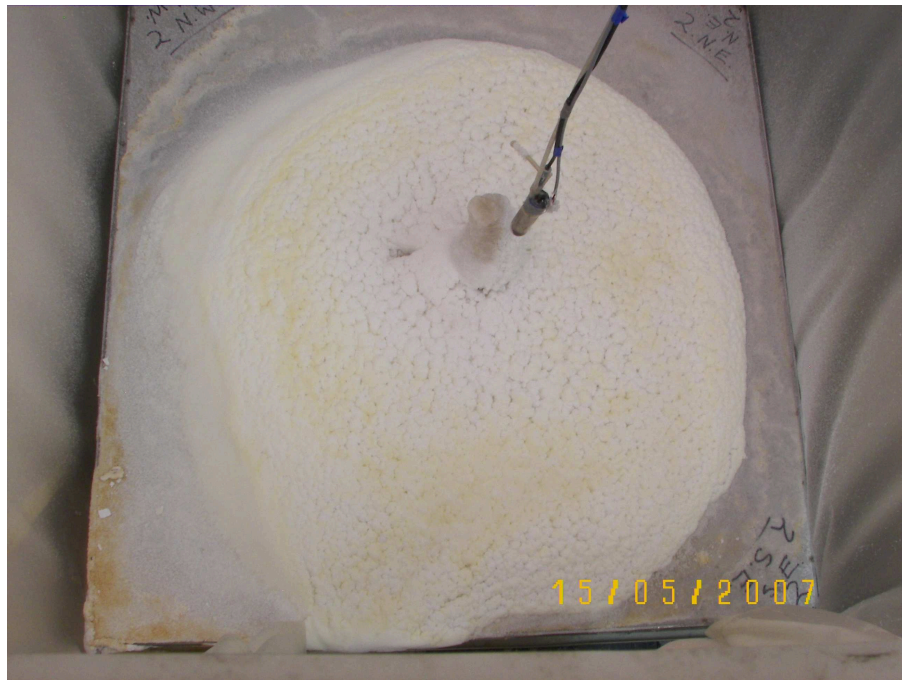
Figure 1.10: Suspended dripper with crystalline deposition across an inclined plate.
