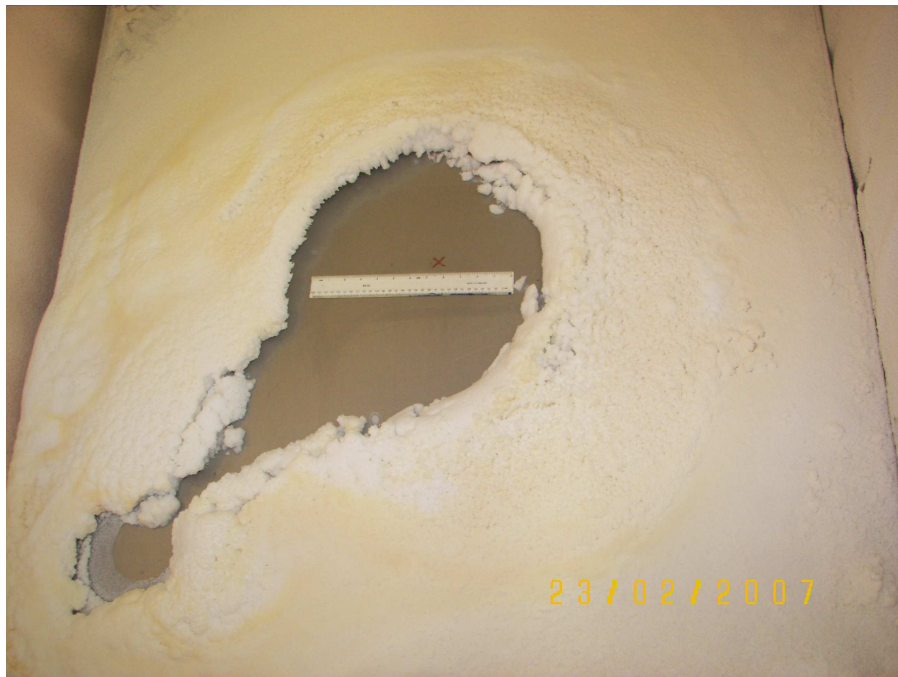
Figure 1.13: 5 Molar sodium nitrate precipitation after 36 day.
