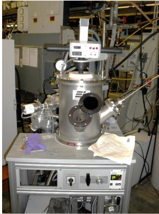
Figure 4.1 Photograph of the arc-melter used in the present study.
