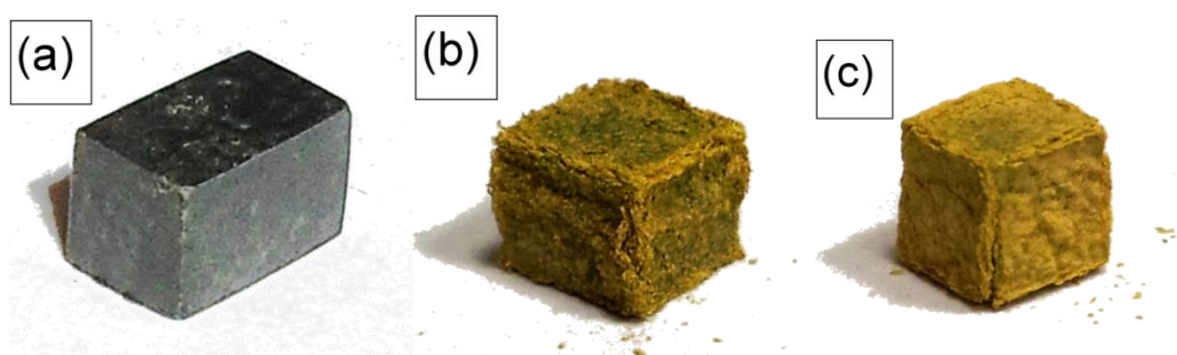
Figure 8.5 Images of samples after oxidation at 800 °C for 100 h. Images show
