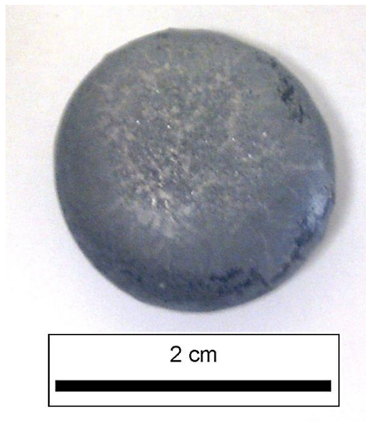
Figure 4.2 Photograph of typical 10 g ingot.
