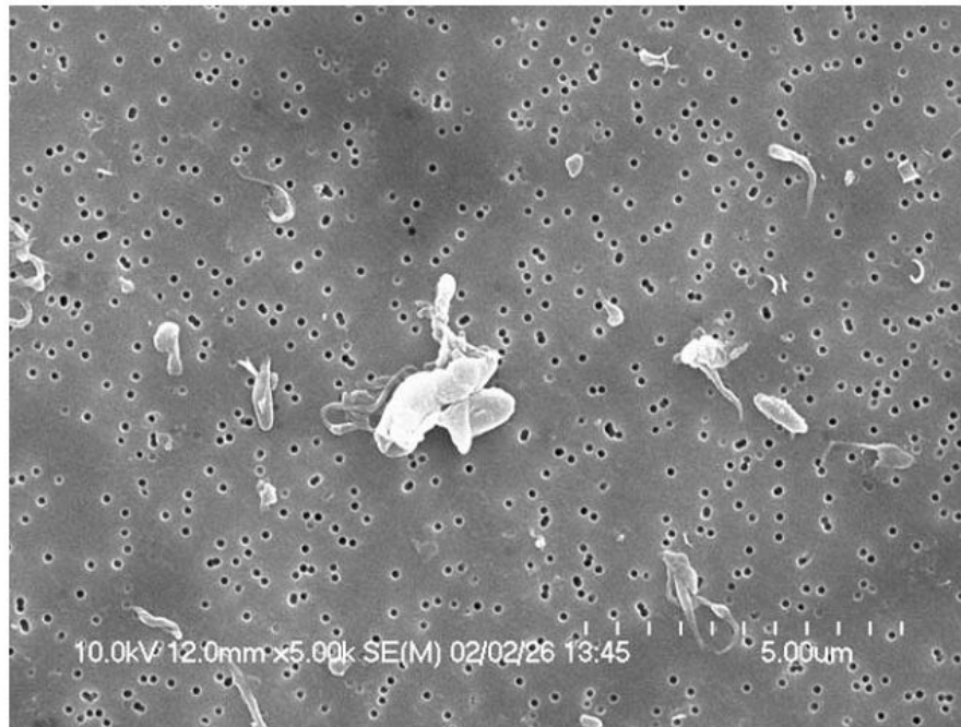
Figure 1.12 Scanning electron microscopy of the polyethylene wear particles (Minoda et al. 2005).
