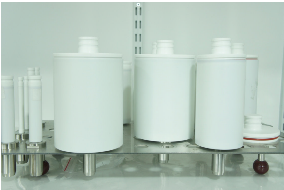
Figure 2.5 Polyethylene methacrylate (PMMA) specimen holders.
