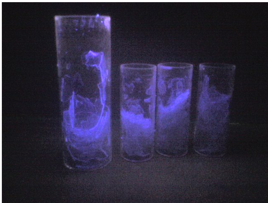
Figure 3.10: Poly(acrylate) Sheets Labelled with 0.1 wt% 9-Vinylanthracene and Containing 4-Bromostyrene Viewed Under UV (365 nm) Light - Containing from left to right; 0 wt%, 0.1 wt%, 0.5 wt% and 1.0 wt% 4-bromostyrene
