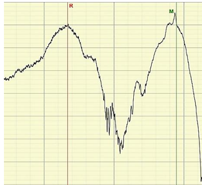
Figure 3.5: Volume lost was measured by tribometer of AZ surface worn under 4N load in water after 24 hours sliding with 0.02 m/s speed.
