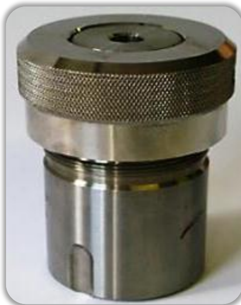
Fig 3.1: Sealed Teflon lined general-purpose vessel
