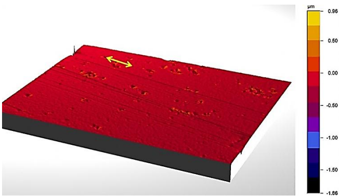
Fig 4.29: AZ sample worn in water under 0.5 N at 0.02 m/s
