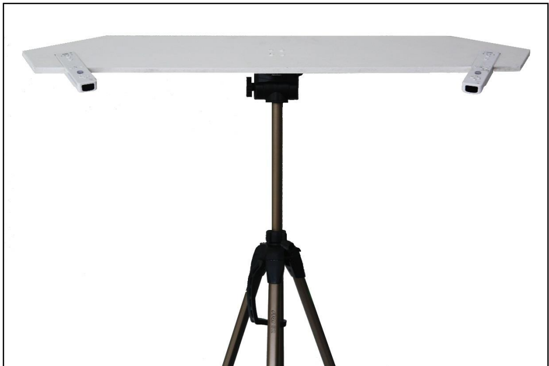
Figure 13. Camera construction on tripod-mounted board
