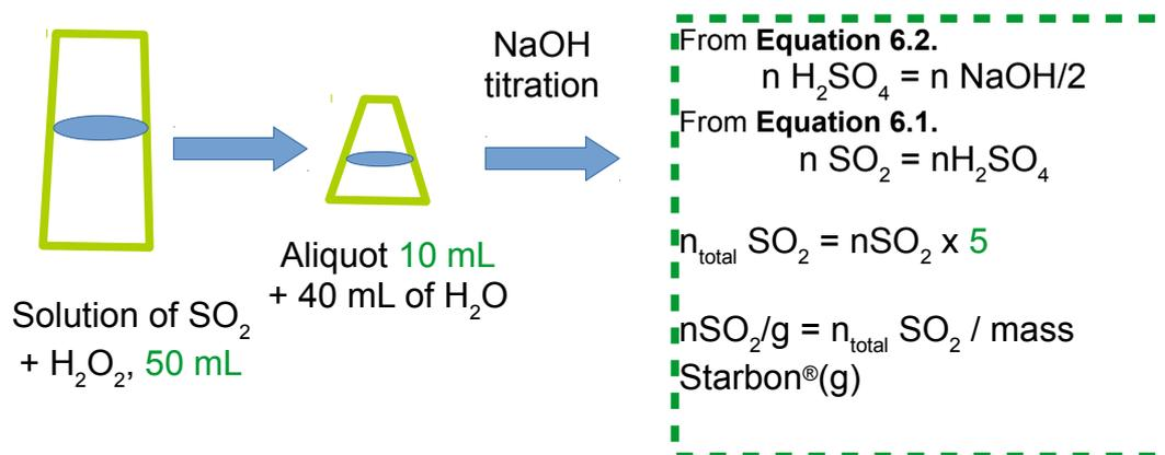
**Figure 6.4.** Schematic representation of the quantification of sulfur dioxide through potentiometric titration
