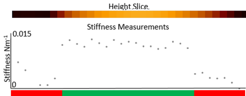
Figure 6.1: Example slice through the centre of a force map, showing a stiffness vs. position graph for the measurement from each point.
