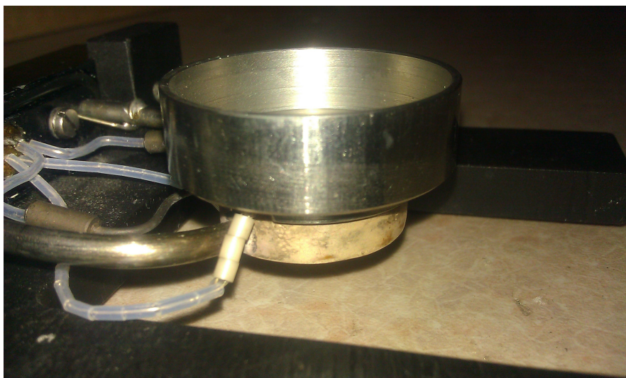
Figure 4.8: Photograph showing the second sample holder mounted on the Linkam heating stage.
