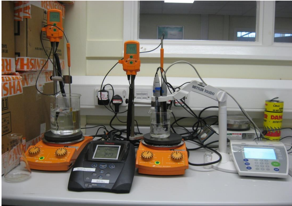
Figure 5-10 : The Mettler Toledo combined conductivity/ion selectivity probe setup used in the bulk measurements and pH meter.
