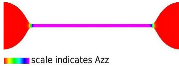
Figure 3.24: Jet profile predicted by the axisymmetric model for fluid parameters Oh = 0.79 , c = 2.37 and De = 94.9 . The colour scale corresponds to the axial component of the structure tensor \mathbf{A} describing dumbbell stretch.
