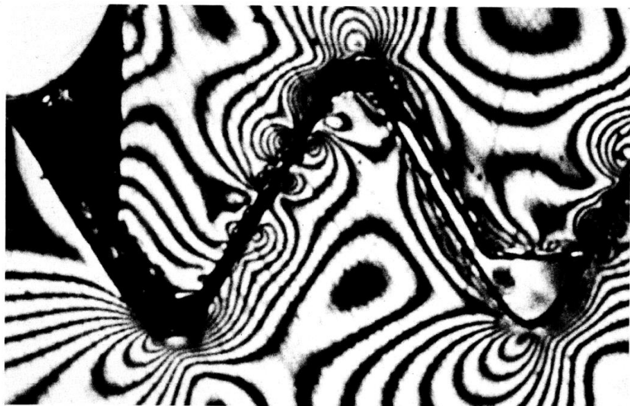
Figure 2.2-12 The x3 multiplied fringe pattern for a thread half a pitch from the loaded face of the nut x26 (copied from [52])
