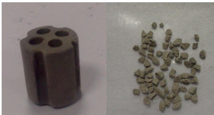
**Figure 3.1** Images of catalyst pellet (left) and catalyst particles (right) used in this project
