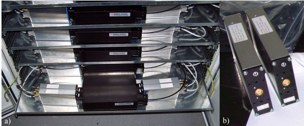
Figure 2.7: JET HRTS polychromator a) optical box and amplifier units as positioned on the shelves within the HRTS cubical and b) amplifier units with the detector lens block detached to reveal APD.
