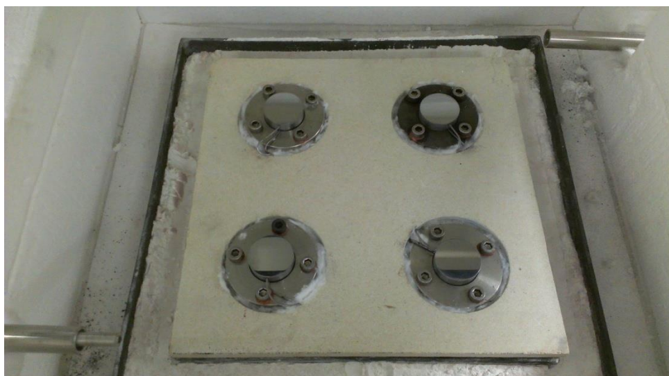
Figure 3.4 Four mild steel samples loaded inside the furnace before start up.
