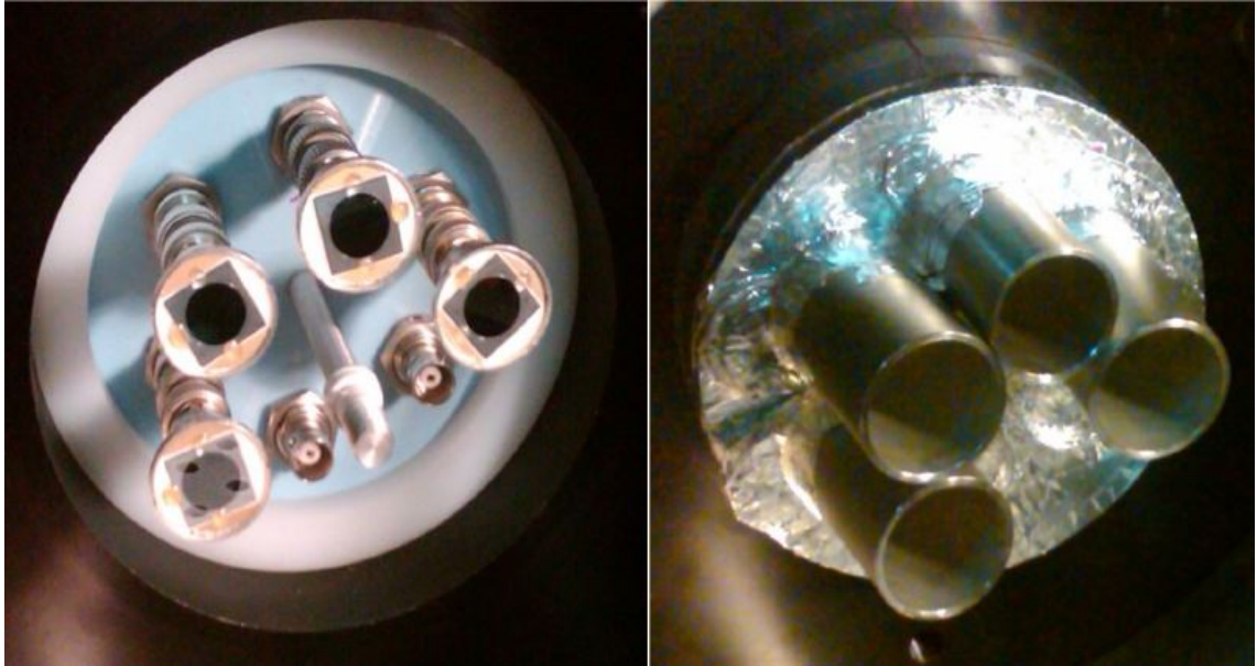
Figure 4.15: X-ray diodes mounted on plastic flange with BNC feedthroughs (left) and covering aluminium housing (right). Each diode covers a 12 mm active region.
