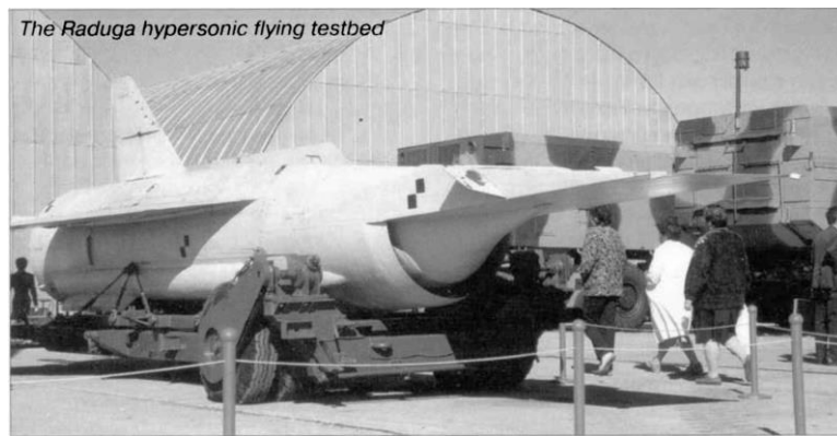
Figure 1.14 Russian GELA/Raduga operational flight test vehicle [21].
