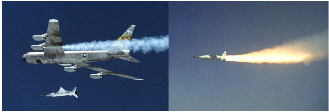
Figure 1.12 The B-52 with hyper-X release and the ignition of Pegasus rocket booster [21].
