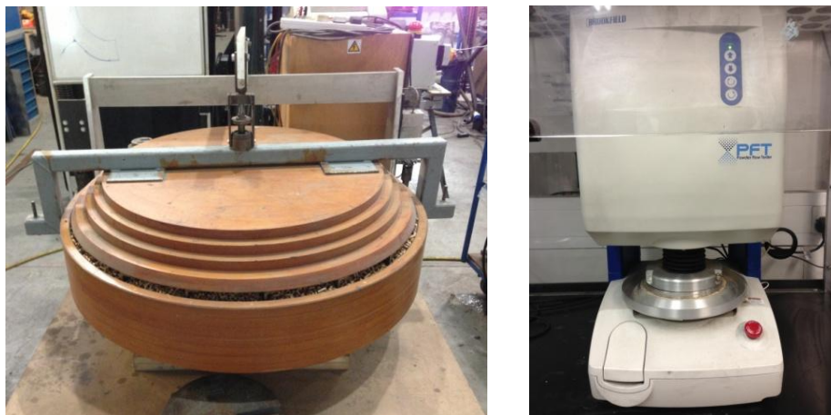
Figure 4-8: Ø1 m annular shear tester (left) and Brookfield PFT (right).
