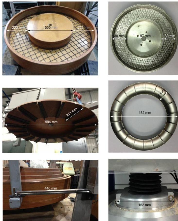
Figure 4-9: Annular shear cell (left) and Brookfield PFT (right). Shear cell, lid and torque sensor (top to bottom).
