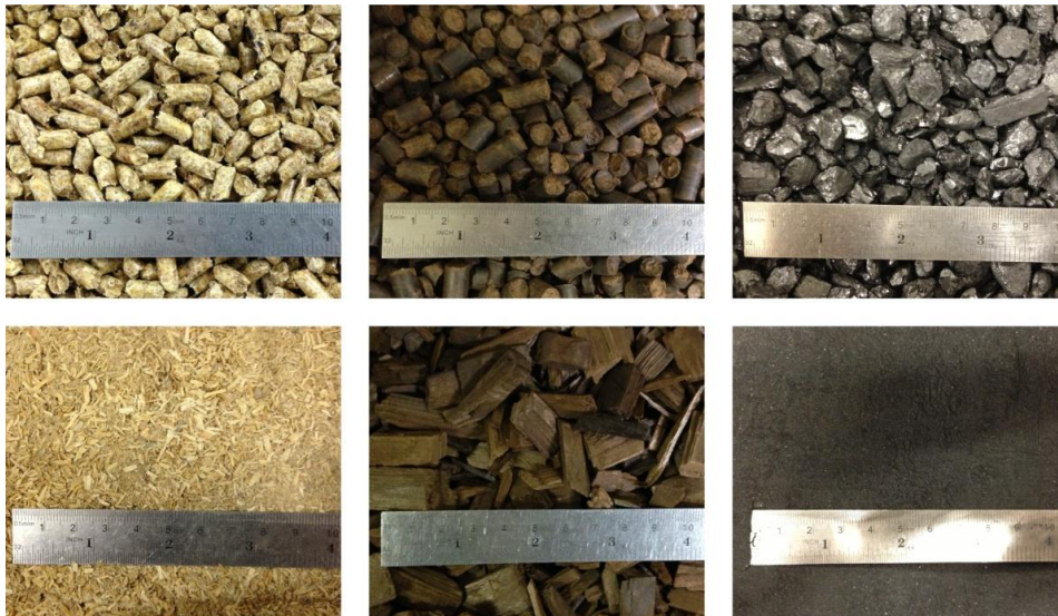
Figure 4-1: Wood pellets, torrefied spruce pellets, coarsely ground anthracite grains (first row, left to right), milled wood pellets, torrefied spruce wood chips and pulverised bituminous coal (second row, left to right).
