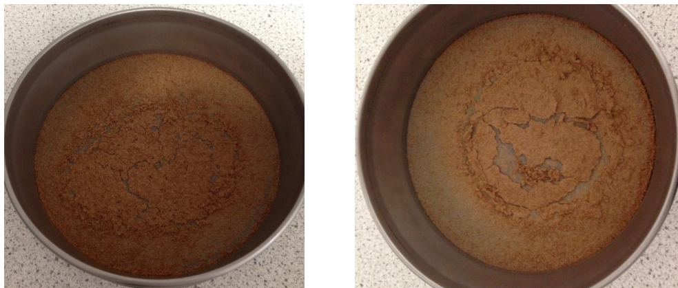
Figure 9: Examples of the impermeable crust formed on the 200 \mu\text{m} sieve.
