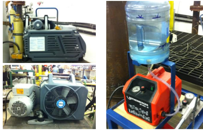
Figure 5-3: Niedermeier three stage compressor (left) and Rothenberger RP PRO III water pump (right).
