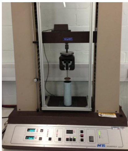
Figure 4-12: Hounsfield tensile tester fitted with a plunger to measure changes in bulk density.
