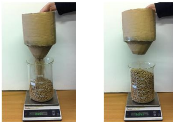
Figure 4-25: Flow of wood pellets from the prototype test hopper.
