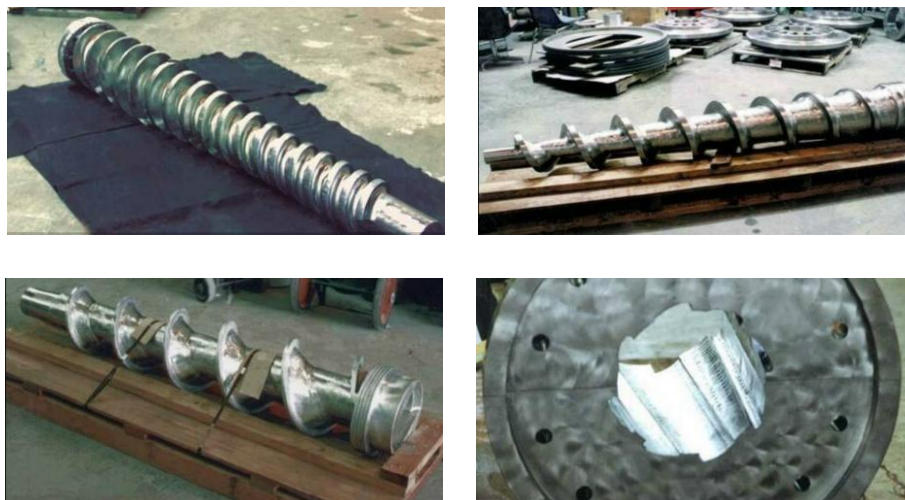
Figure 2-10: Screw types available from MST Corporation (MST, 2010).
