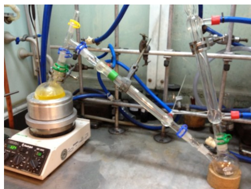
Figure 63: Steam distillation set-up used for D -limonene purification (originally in colour).
