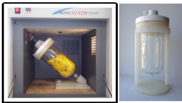
Figure 102: Milestone ROTOSYNTH equipment containing WOP for the purpose of the D -limonene microwave extraction –left and 1 L Pyrex® glass reactor –right (originally in colour).
