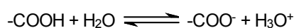
Figure 48: Influence of pH on the dissociation equilibrium of free carboxyl acid functionalities.
