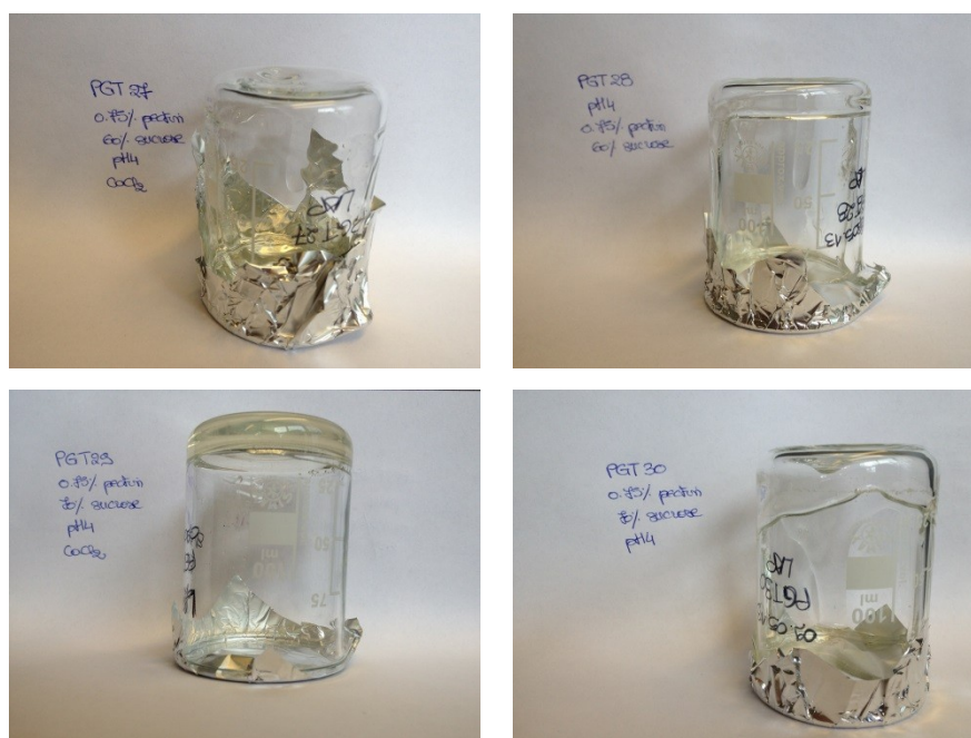
Figure 52: End-result of gel test PGT27, PGT28, PGT29 and PGT30 with pectin P0023 using the Lofgren protocol (originally in colour).
