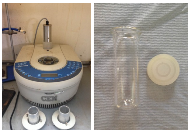
Figure 100: CEM Discovery SP microwave equipment - left and CEM Discovery 35 mL Pyrex® vial with corresponding silicon cap-right (originally in colour).
