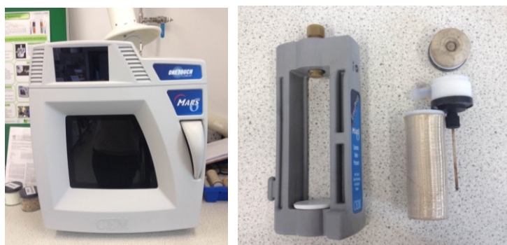
Figure 101: CEM MARS 6 equipment -left, and control vessel & support -right (originally in colour).
