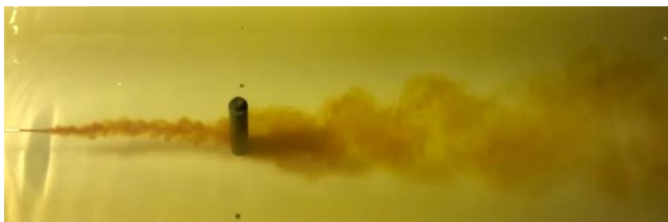
Figure 5-18 – Vortex shedding behind 16mm diameter support structure ( Re = 4919 ).
