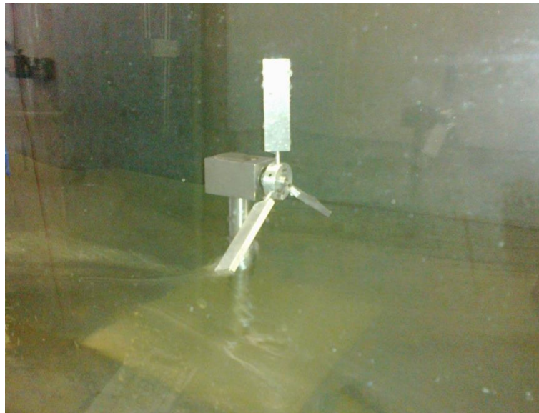
Figure 3-20 – Initial turbine model.
