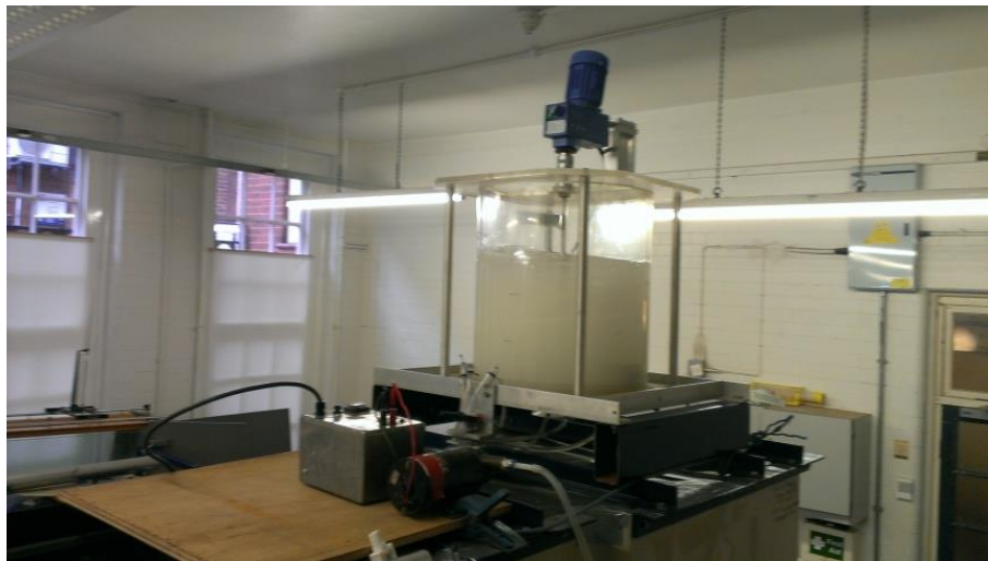
Figure 3-15 – Seeding mixing tank and injection system.
