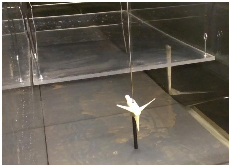
Figure 3-17 – Transparent surface smoothing plate in situ.
