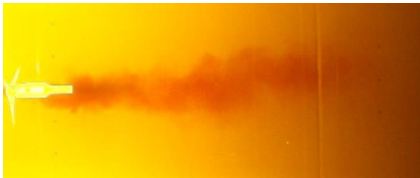
Figure 6-16 – Wake drift observed in dye injection results.
