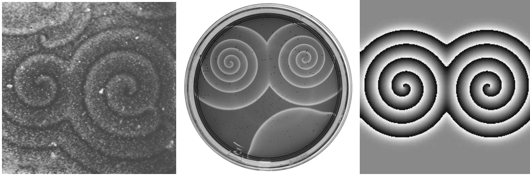
Figure 4.1: Spiral waves in a biological and a chemical system. Left panel: chemotactic movements of amoeba population reproduced from [BiophysikBildergalerie] . Centre panel: the Belousov–Zhabotinsky chemical reaction reproduced from [ChemWiki] . Right panel: numerical solution of the two-dimensional CGLE with phase of the complex amplitude encoded in greyscale.
