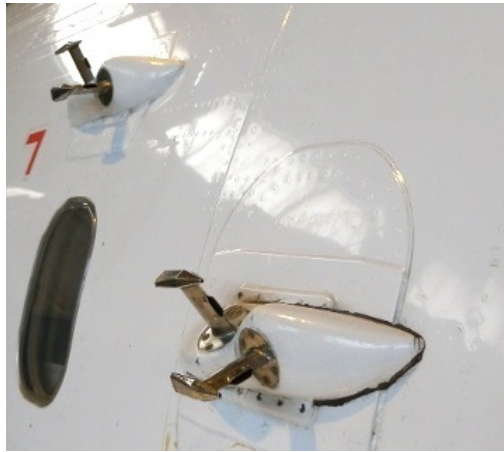
Figure 4.9 Modified Rosemount housings on the port side of the aircraft.
