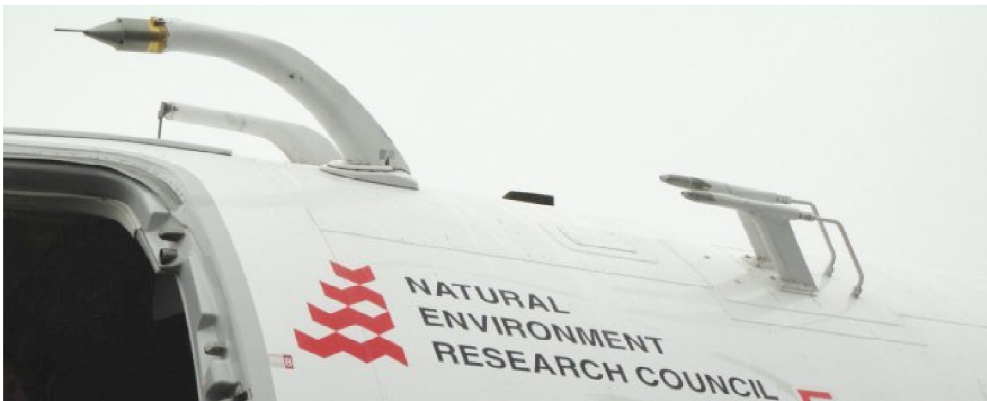
Figure 4.11 Photograph indicating the position of the LTI on the BAe-146 aircraft ( foreground ), including ( right ) the isokinetic inlets which sample to the filter system and ( behind ) the trace gas sample line.
