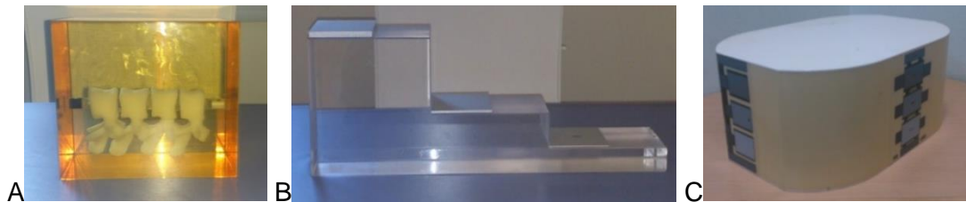
Figure 11: Phantoms for the calibration of the DXA device Hologic anthropomorphic spine (A), step (B) and European spine (C) phantoms
