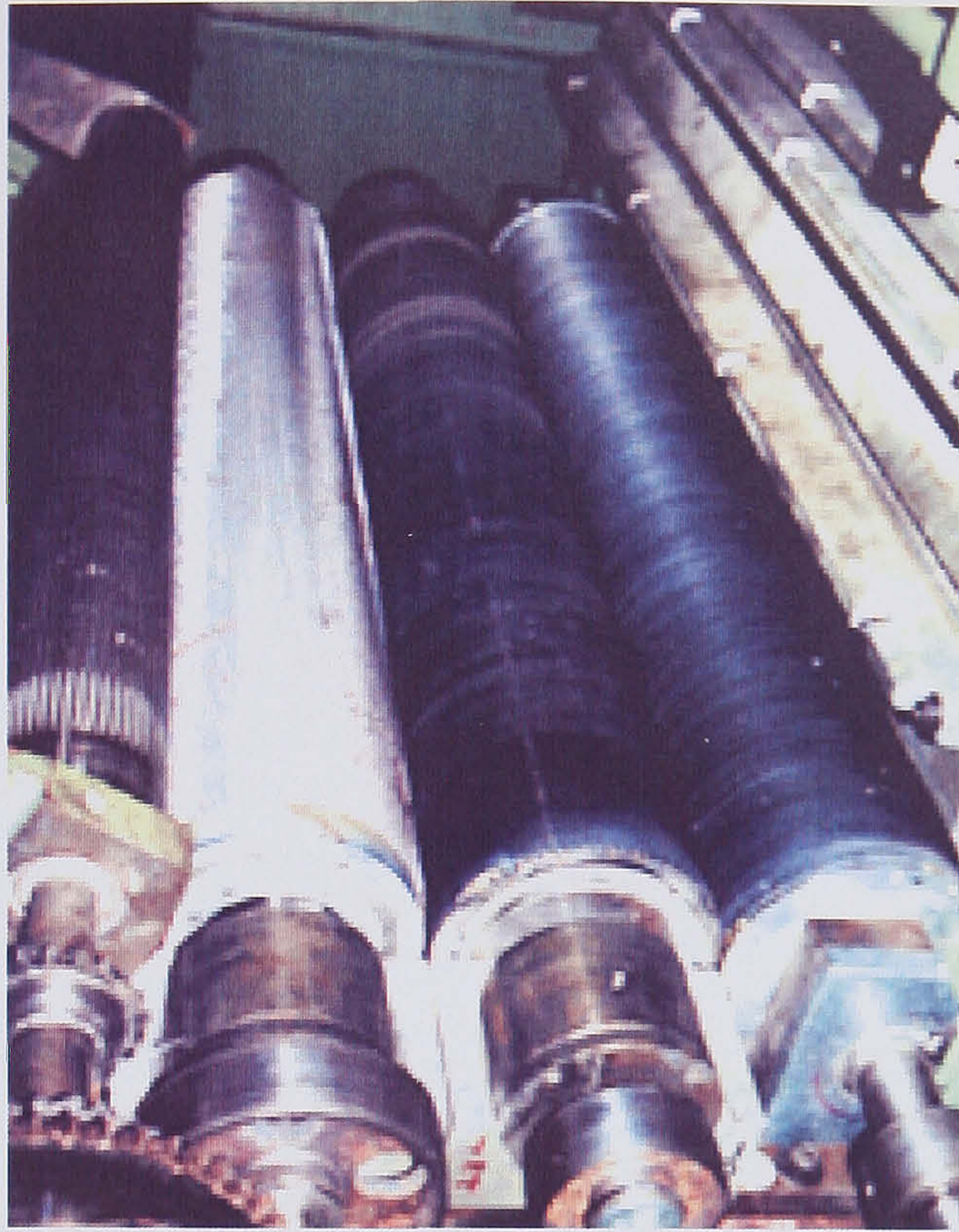
Figure 2.13 – Roller arrangement in triple licker-in unit on the card (without enclosures)
