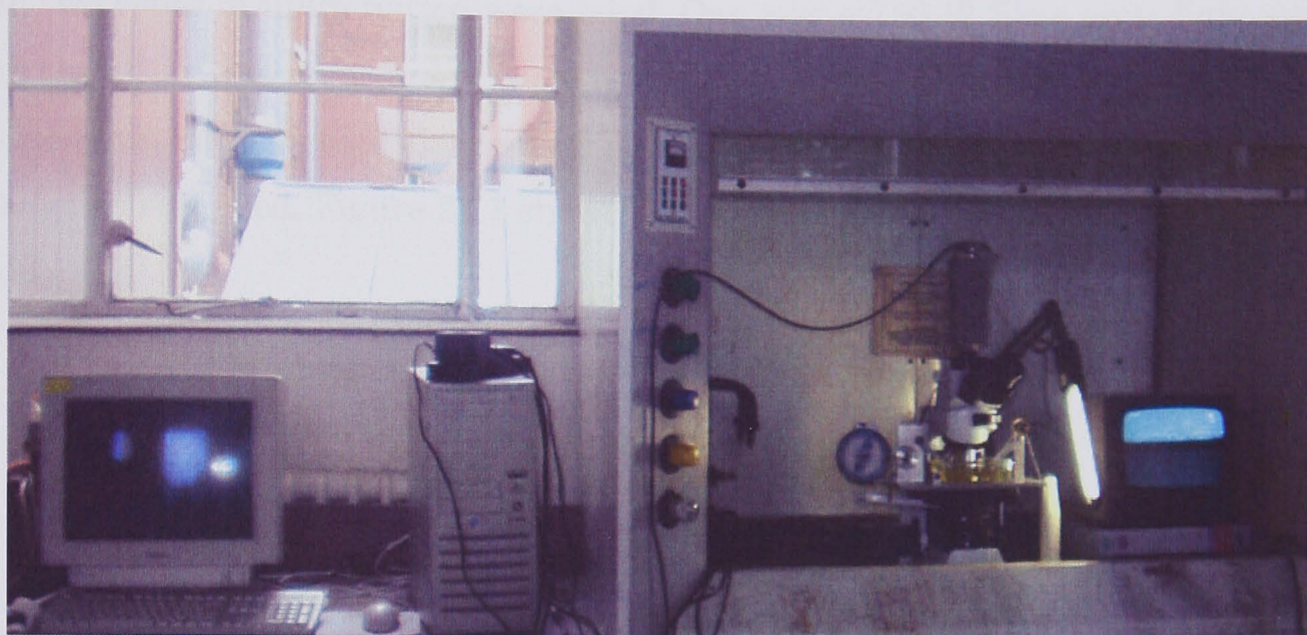
Figure 2.10 – Complete tracer analysis arrangement showing fume cupboard, computer and connections
