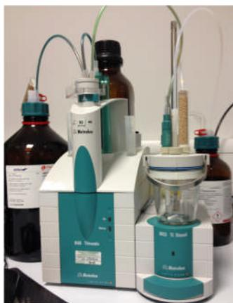
Figure 3.4-14. Karl-Fischer Metrohm Titration equipment for moisture determination in liquid samples
