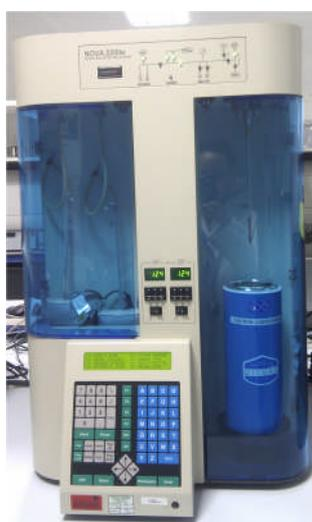
Figure 3.4-4. BET surface area and pore size analyser: Quantachrome NOVA 2200e
