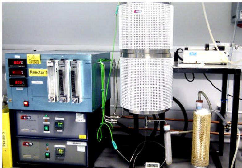
Figure 3.3-2. Assembled and main parts of the pyrolysis/gasification reactor.
