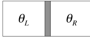
Figure 1.1: A Josephson junction, which consists of two superconducting regions separated by a thin insulating barrier, or in general, a ‘weak link’. The superconductors on the left and right of the junction have condensate phases \theta_L and \theta_R , respectively.
